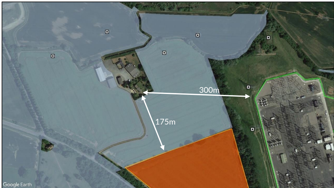
Figure 6 Minimum distance between BESS 2 and the nearest dwelling, as well as the relative location of Grendon Substation
